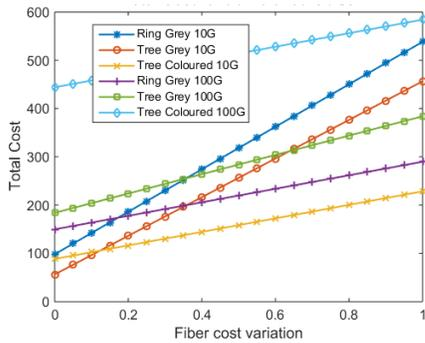
Fig. 11. Total cost network vs. fiber cost variation for a total traffic of 50 Gbit/s
