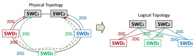
Fig. 3. Physical and logical topology for coloured ring deployments
