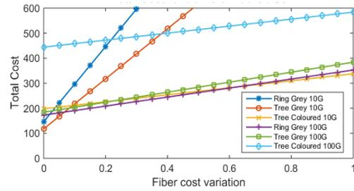
Fig. 12. Total cost network vs. fiber cost variation for a total traffic of 200 Gbit/s
