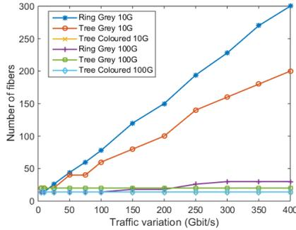
Fig. 10. Number of needed fibers for each deployment vs network traffic variation
