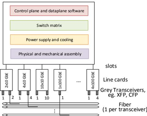
Fig. 6. Node architecture for dark fiber deployments
