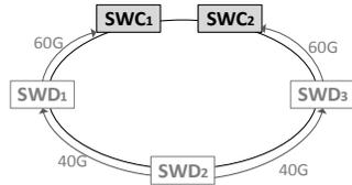
Fig. 1. Example of metro ring topology with no optical layer
