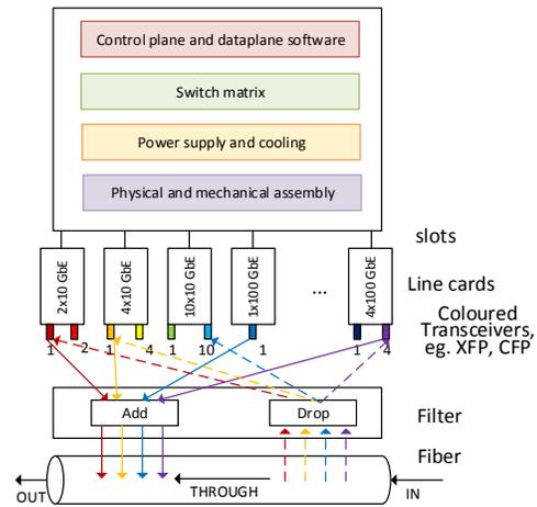
Fig. 7. Node architecture for passive optical deployments (coloured transceivers)
