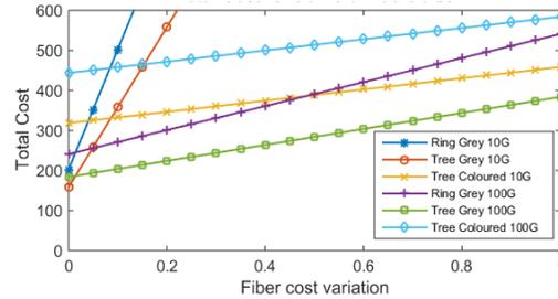
Fig. 13. Total cost network vs. fiber cost variation for a total traffic of 400 Gbit/s
