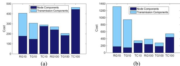
Fig. 15. Comparison of component costs for each topology for traffics of 300 Gbit/s when considering (a) cost fiber of 0.1 (b) cost fiber of 0.5
