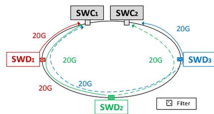
Fig. 5. Example of passive optical metro architecture
