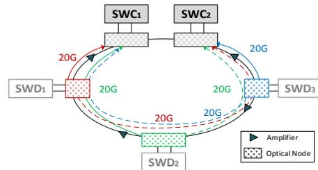
Fig. 4. Example of CWDM/DWDM metro architecture with optical nodes
