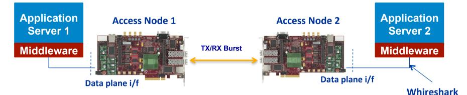
The burst size threshold is set to 6400 bytes (50 packets). Based on the PCAP file captured at Server 2, the burst is correctly transmitted.
