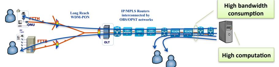
Distributed cloud approach: Multiple multipurpose servers located in metro and core nodes
